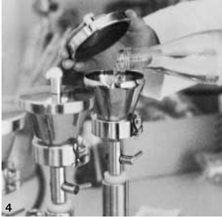
Pouring the liquid to be examined into the funnel
