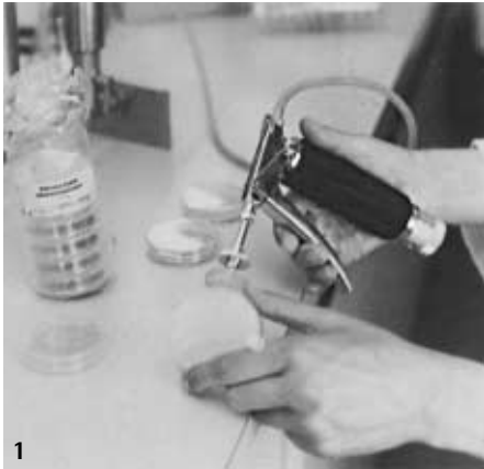
1 Prewetting Nutrient Pad Sets with sterile water (using the Sartorius Dosing Syringe, as pictured here, or a pipette)
